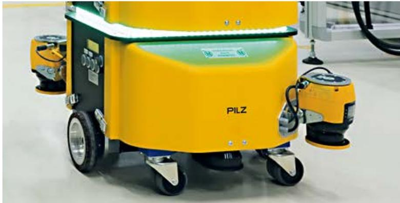
In this example, the AGV is moving in an aisle at one side of a production hall to deliver material needed for a machine. The aisle is wide enough to be assessed as a normal “operating zone” with the AGV operating at full operation speed, since clearances of 500 mm or more to each side are achievable.
