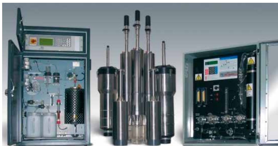
Figure 2: Types of online TOC analysers - on the left a high temperature oxidation analyser, in the middle some UV absorption analysers, and on the right a chemical oxidation analyser.
