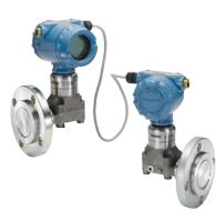
Featuring best-in-class performance and measurement stability, the Rosemount 3051S Electronic Remote Sensor (ERS™) System is engineered with flexible, digital architecture. The ERS System calculates differential pressure electronically using two pressure sensors linked together with an electrical cable. Easy to install, this safety-certified system is engineered for faster response time than traditional systems, providing you with exceptional performance in the brew kettle.
