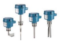
The Rosemount 2500 Solids Switch range offers the complete choice of point level measurement for bulk solids. Four different technologies are available. Rotating paddle, vibrating rod, vibrating fork, and capacitance. The switches provide flexible measurement fo powders, grains, and pellets and their compact size makes them ideal for installation in all sizes of vessels and silos.
