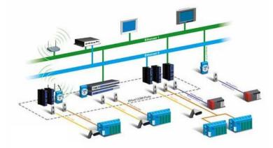
The COM port redirection software is installed on the computer somewhere on the LAN. The remote devices are addressed as virtual COM (VCOM) ports. The entire system behaves, as far as the serial devices and host computer are concerned, as if there is a hard-wired direct connection between the serial device and the COM port on the computer. This is made possible by serial tunneling. Serial data is encapsulated in IP packets and transported over the Ethernet network, just
