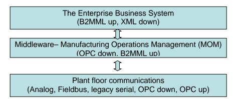
The venerable Purdue model of manufacturing has been compressed to the three layers shown here. There is the plant floor, and all the communications that occur there. There is the MOM system, which connects the plant floor to the manufacturing business systems, and to the enterprise business system.
