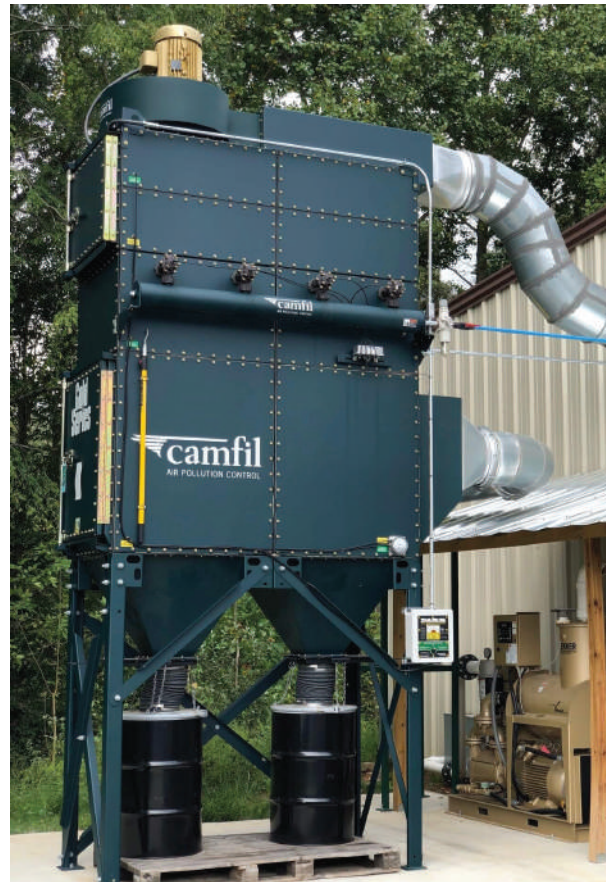
Eight-cartridge dust collector captures laser cutting fumes from an automated tube cutting application.
